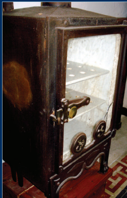
Vintage oven for heat sterilization by Dylan Said. The temperature being raised enough and prolonged adequately to kill all bacteria and spores.
